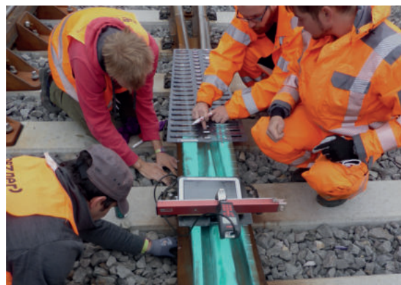
Fig 7. Voestalpine staff checking the turnout crossing geometry at Pfaffstätten prior to the in-track noise measurements being recorded.
