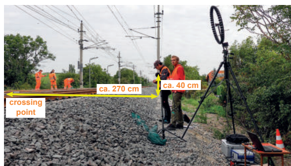
Fig 8. Setting up the measurement equipment to record the noise of passing trains during the field trials at Pfaffstatten.
